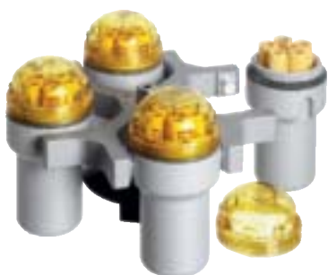
rotor No. 1624 with carriers No. 1381 and lids No. 1382 with bio-containment 5)
