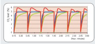
Precisely tuned sensor and software result in fast recovery of CO<sub>2</sub> without overshoot. This ensures uniform CO<sub>2</sub> levels even with frequent incubator door openings.\*
