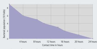
Esco **ISOCIDE**™ is an antimicrobial inhibitor that eliminates 99.9% surface bacteria within 24 hours of exposure. Isocide is integrated into the coating and cannot be washed out or diminished by repeated cleaning.
