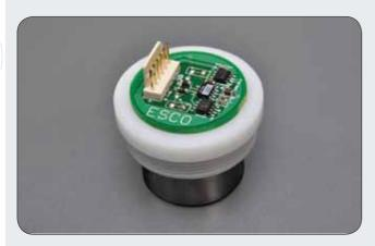
Esco TC  $CO_2$  sensor's operating principle relies on a resistor as a heater and two thermocouples as a sensing element for the  $CO_2$  gas. Accurate sensing is made possible by the porous cap on the eye of the sensor probe.
