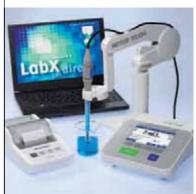
Upon endpointing SevenCompact™ allows multiple archiving options: the data can be stored, printed or transferred to LabX direct. Any combination of these three options is possible giving you total flexibility.
