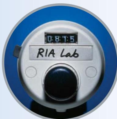
● It can be readjusted when tested according GLP and calibrated for liquids with a different density than water. According to EN ISO 8655 the readjustment for more safety and transparency is sealed.
